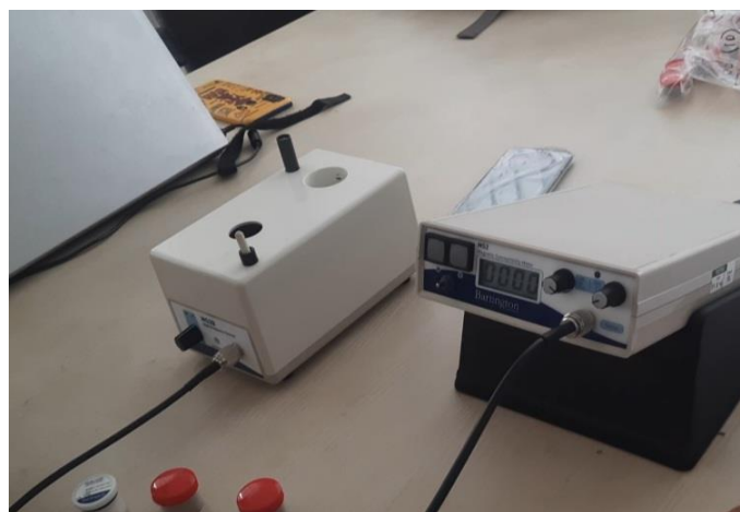
Figure 3 Bartington Magnetic Susceptibility Meter, Geophysical Laboratory, Asutosh College, Kolkata, West Bengal.
